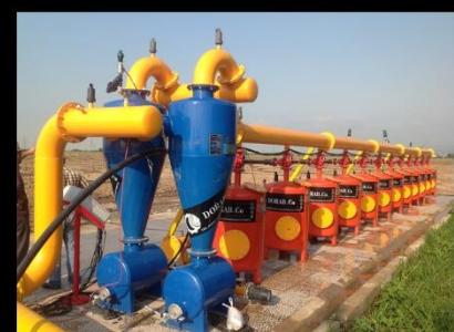
Hydro cyclone Filter (Sand Separator)
